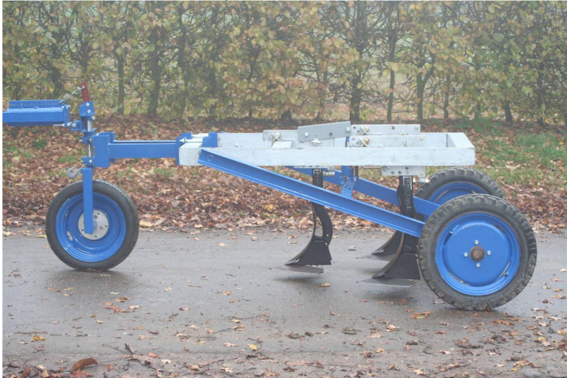
Cultivator prototype from 2008 for cultivation with workhorses, but no traditional plow. Project “Humussphäre”
